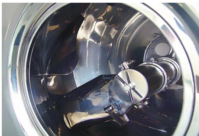
Internal structure of coating drum
