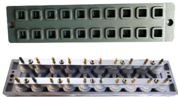
Metal mold with release pin on the back
